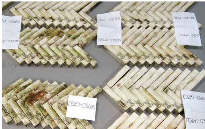
Teknos tests in Malaysia are based on the standard L-joint method as defined in EN 330.
